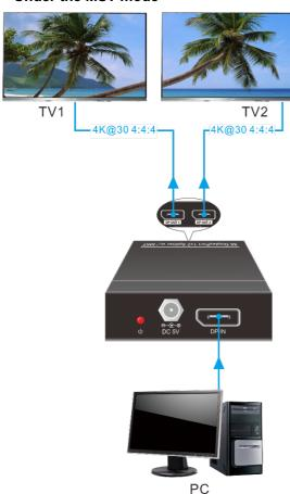
**Note:** Output resolution: 1.two output ports support 4K@30Hz (Max) simultaneously; 2.one output port supports 4K@60 Hz, another output port only supports 2K.
