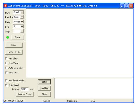
Please set the parameters of COM number, bound rate, data bit, stop bit and the parity bit correctly, and then you are able to send command in Command Sending Area.
