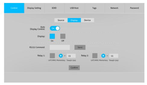
Auto Display Control: Enable or disable the auto display control mode. In auto display control mode, the unit will automatically perform the following operations.
