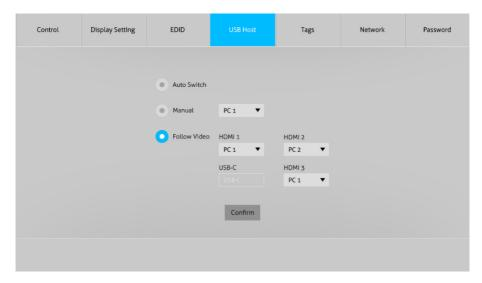
The system provides USB HOST PC 1, PC 2 or USB-C to be selected, and it provides USB Type-A ports for connecting USB devices (e.g. mouse, keyboard, etc.) used to control the selected USB HOST. The USB HOST can be switched in this tab.
