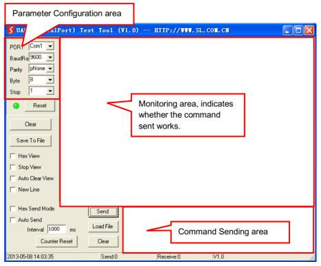
Please set the parameters of COM number, baud rate, data bit, stop bit and the parity bit correctly, only then will you be able to send command in Command Sending Area.
